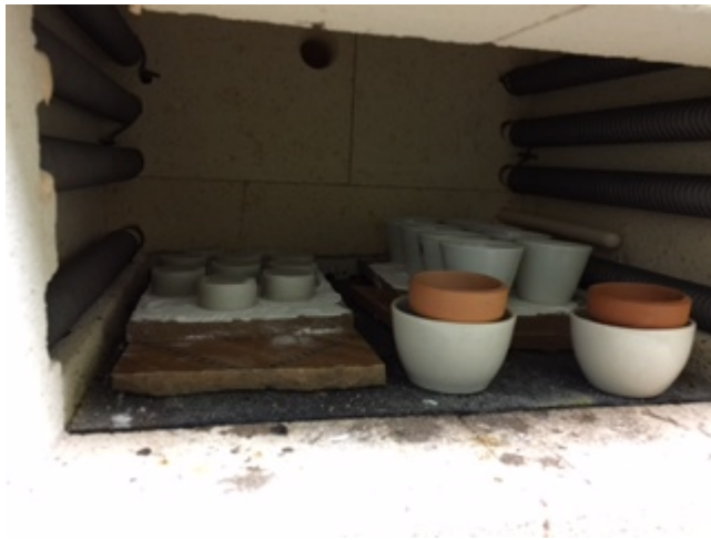
Pressed and unpressed samples in furnace
