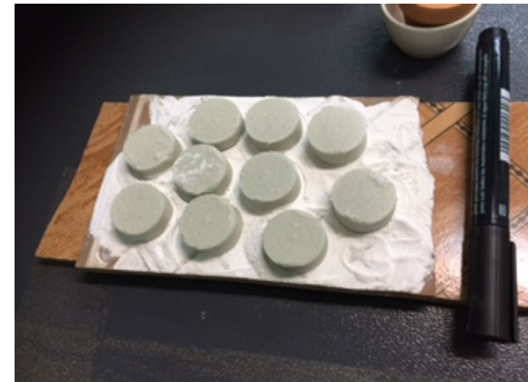
Pressed samples after sintering
