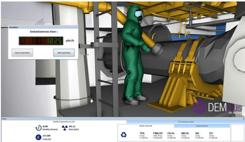
Dose rate computation at the place of work obtained with DEMplus® for nuclear
